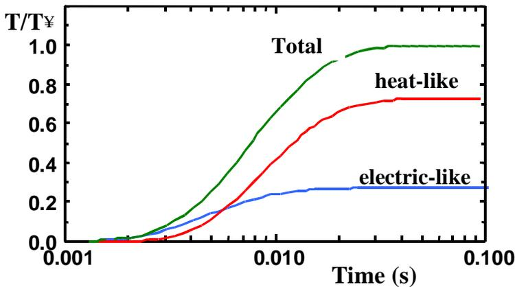
Figure 4: Temperature vs. time response for a flash diffusivity measurement on a hypothetical metal 1 mm thick with  $\gamma_c \sim 2$  and  $\gamma_L \sim 2$ .
