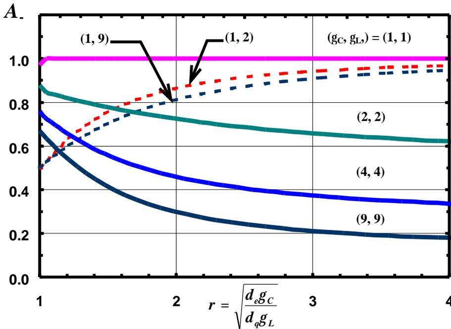
Figure 3: Amplitude of the 'heat-like' response as a function of the diffusion constants neglecting coupling ( $d_e$  and  $d_q$ ) and the magnitude of the coupling ( $g_c$  and  $g_L$ ).
