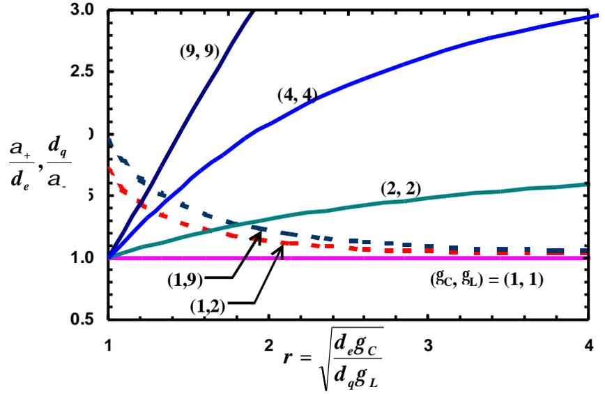
Figure 1: Actual diffusivity values  $a_+$  and  $a_-$  as functions of the diffusion constants  $d_e$  and  $d_q$  neglecting coupling and the magnitude of thermoelectric coupling ( $g_c, g_L$ ).
