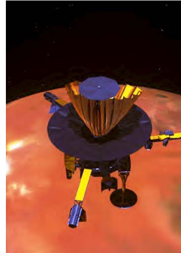
Figure 2. Galileo spacecraft over Io. One of the two GPHS-RTGs is shown at the bottom. (JPL)
