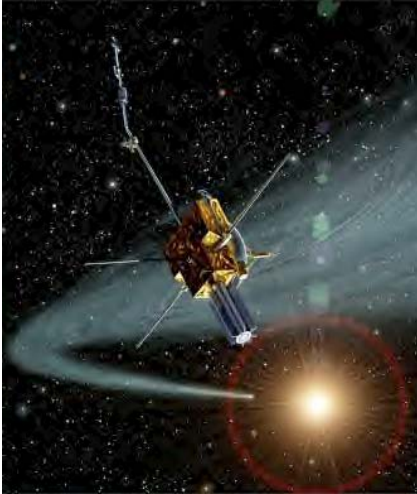
Figure 1. Ulysses spacecraft in tail of Comet Hyakutake. The single GPHS-RTG is shown at the bottom. (ESA)
