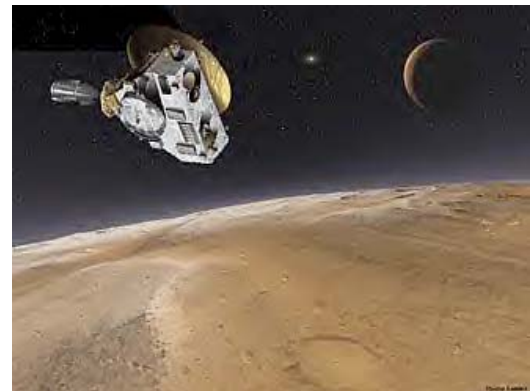
Figure 4. New Horizons spacecraft shown flying by Pluto with satellite Charon in the background. The single GPHS-RTG is shown mounted on the left side of the spacecraft. (JHU/APL and SwRI)
