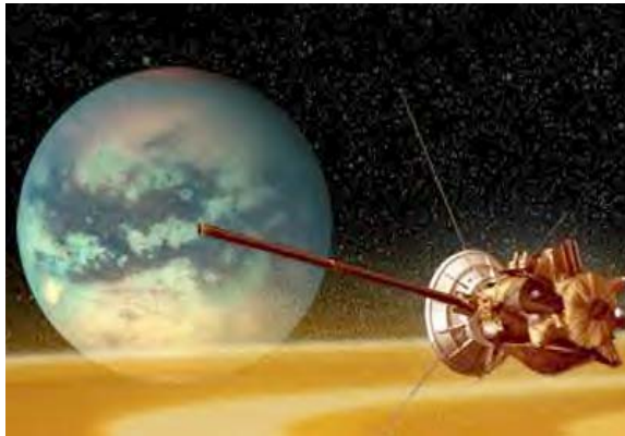
Figure 3. Cassini spacecraft over Saturn's rings with Titan, Saturn's largest moon. One of the three GPHS-RTGs is shown near the top of the spacecraft. (NASA/JPL)
