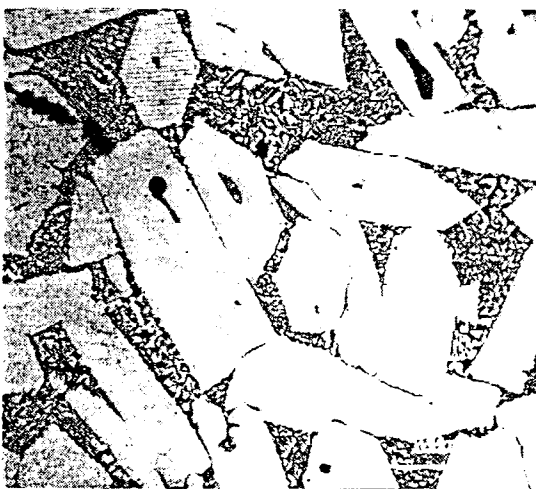
Figure 5. Eutectic composition alloy showing the intimate mixture of \text{IrSi}_{-3} (light) and Si (dark).
