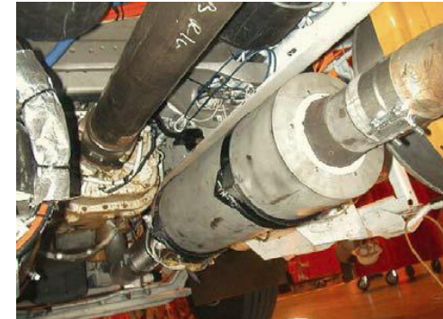
1 kW TEG on a Kenworth Truck [Hi-Z]
