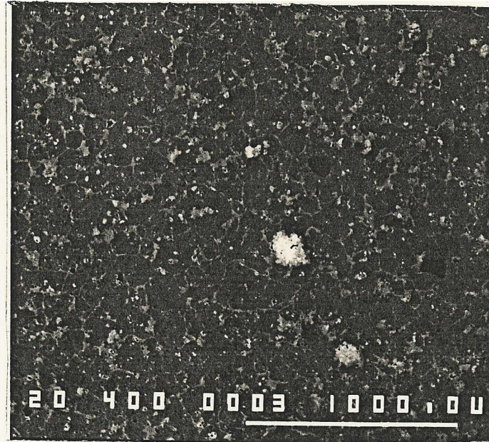
FIGURE 13. Micrograph of T-428, Hot-Pressed SiGe/GaP, After Various Heat Treatments (40x).
