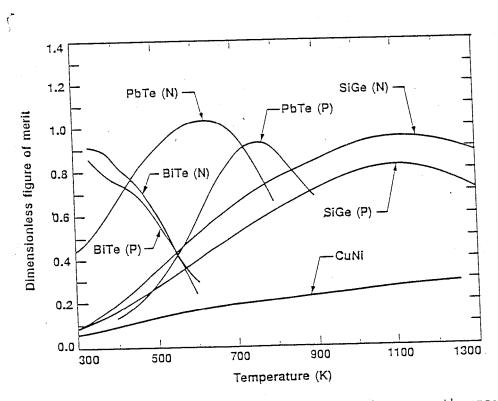
re 2 The dimensionless figure of merit for several common thermos materials peak at values near ZT=1. CuNi, a metallic alloy for comparison, has a much lower figure of merit value.
