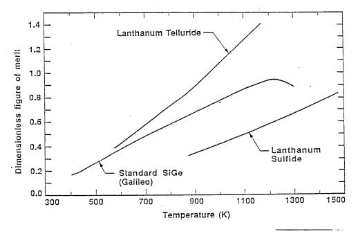
! The figure of merit of advanced rare-earth chalcogenides base lanthanum telluride have recently surpassed the ZT=1 values t of prior thermoelectric materials by a significant margin.
