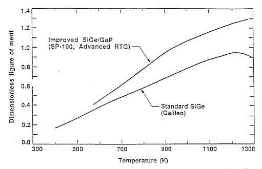
Recent improvements in n-type silicon-germanium alloys doped w gallium phosphide have achieved figure of merit values 30% hig than typical of standard silicon-germanium alloys currently ut in radioisotope thermoelectric generators.
