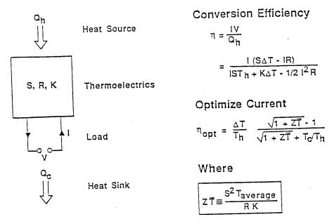
1 The optimized efficiency of a thermoelectric device depends of the dimensionless figure of merit, ZT, and approaches the Carlimit for large figure of merit values.
