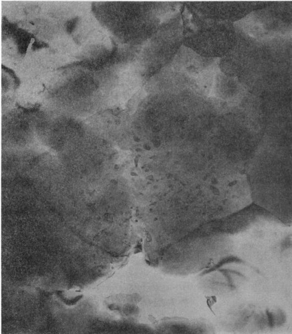
Figure 6-6. TEM Micrograph of Sample ITM-232 Showing Spherical Precipitates within Grains and on Grain Boundaries (20KX Magnification)
