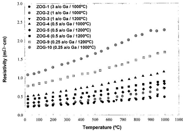
FIG. 2. Temperature dependence of the electrical resistivity of Ga-doped ZnO.
