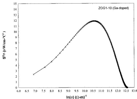
FIG. 5. Predicted ( $S^2\sigma$ ) at 1000 °C of Ga-doped ZnO.
