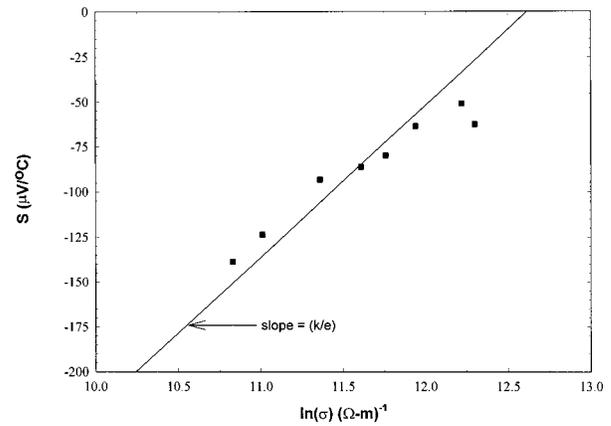
FIG. 4. Jonker plot of Ga-doped ZnO samples at 1000 °C.
