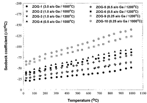
FIG. 1. Temperature dependence of the Seebeck coefficient of Ga-doped ZnO.
